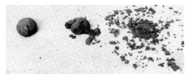
head height onto a hard surface will indicate general characteristics. If the ball of soil explodes, it is too sandy and cannot be used as a building material. If it flattens slightly and does not crack, it will probably have too much clay and must be thinned by adding sand. A good soil will retain its shape and crack only slightly after being
