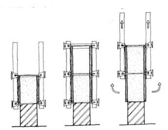
Above: Sliding Formwork for Rammed Earth
