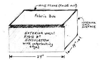
Above: Fabric box with one side of rigid insultion for building segmented earth wall.
