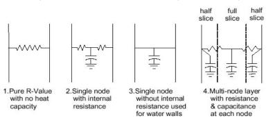
either an R-value or a specified material described by its thickness, specific heat, density, and conductivity. In this way, walls of almost arbitrary complexity may be treated. Additionally, if the walls are part of an exterior surface and the user wishes to determine the effects of solar energy on the wall, the azimuth, absorptance, and parameters for shading can also be specified.
