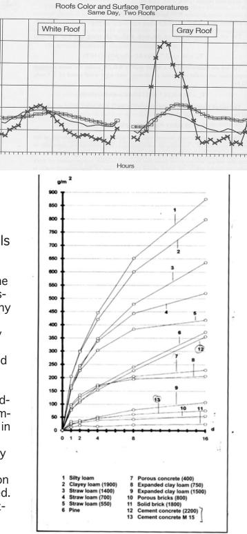
1.4-4 Absorption curves of 11.5 cm thick interior walls with two sides exposed at a temperature of 21°C after a sudden rise in humidity from 50% to 80%
