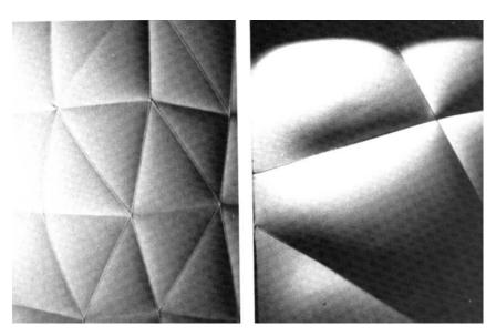
Above: Lost fabric formwork for poured earth.
